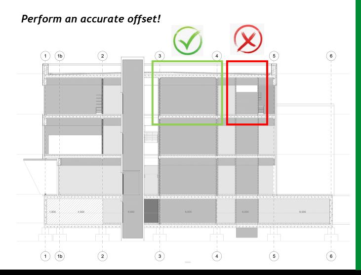
It is important to check that the boundaries of the spaces touch all the enclosing surfaces both **laterally and superiorly**.
