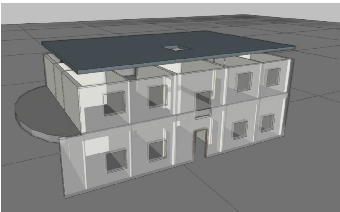
Figure 85. 3D view of the model converted in IFC Builder: The curved wall is not present.
