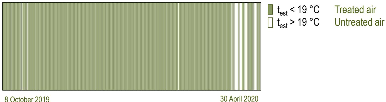
The air must be conditioned for 96% of the activation time, so a constant supply temperature of  $19^{\circ}\text{C}$  has been considered
